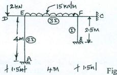
Analyse the continuous beam shown in Fig Q3 by moment distribution method. Sketch the BMD, SFD and Elastic curve, EI constant. (20 Marks)
